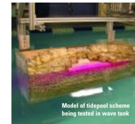
Model of tidepool scheme being tested in wave tank
